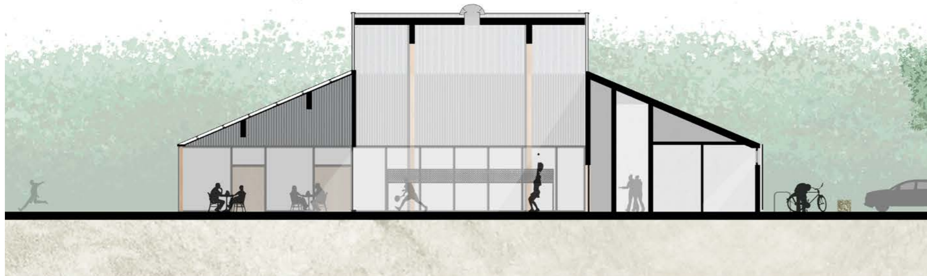
Fig 47: Cross sections showing general arrangement and hierarchy of spaces and clerestory / lantern
