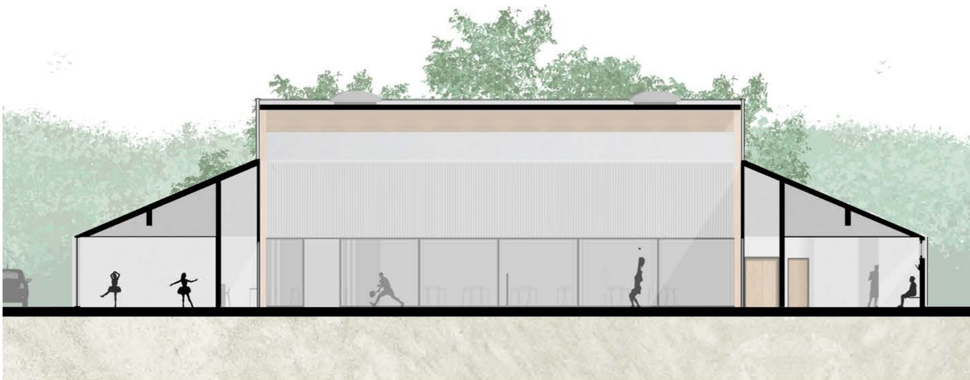
Fig 48: Cross sections showing intervisibility between inside / outside spaces and opportunities for perimeter service zone
