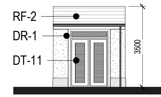
12 Gas Meter - South Elevation 1:100
