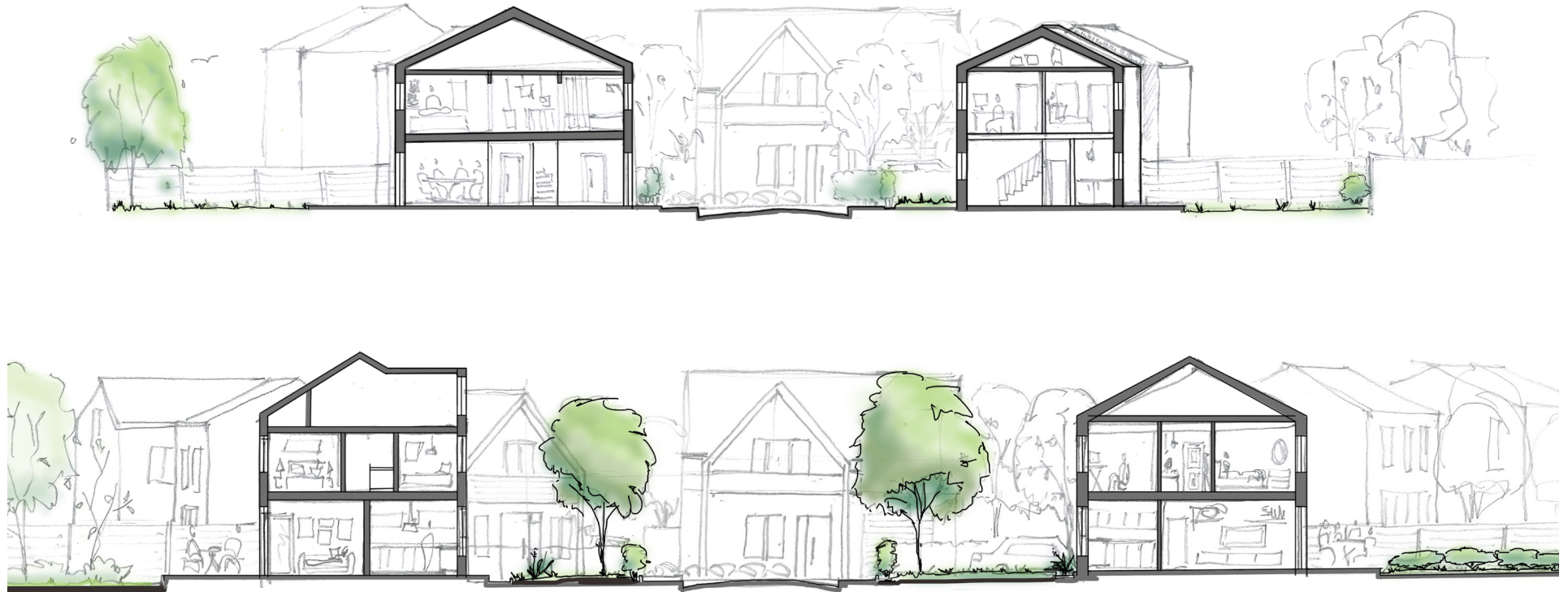
Figure 8. Cross section of the street showing the increase of amenity space between the buildings as progress to the extremities of the site.
