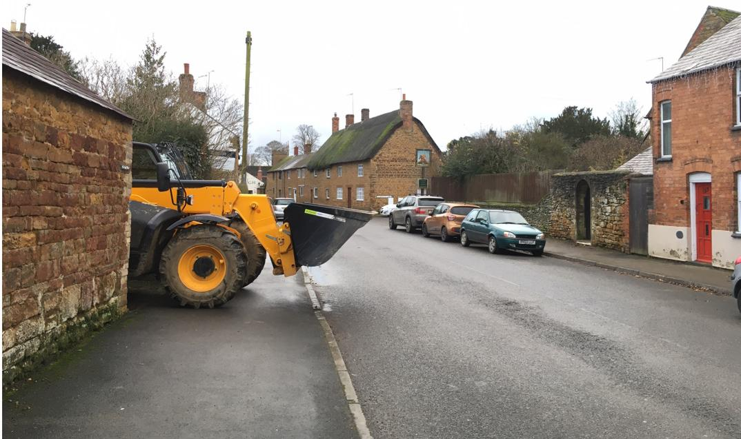
When the cab of the machine is in a sighted position the sight lines are still poor and as a result the boom of these machines is often lifted, against best practice guidelines, to improve the angles. Operation of the machine to gain entry and exit in this way increases the risk to road users in several ways and also damage to over head lines (Fig 13,14).
