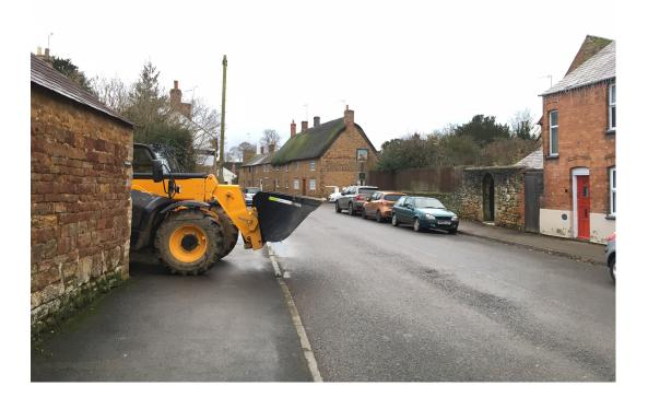
When the cab of the machine is in a sighted position the sight lines are still poor and as a result the boom of these machines is often lifted, against best practice guidelines, to improve the angles. Operation of the machine to gain entry and exit in this way increases the risk to road users in several ways and also damage to over head lines (Fig 13,14).
