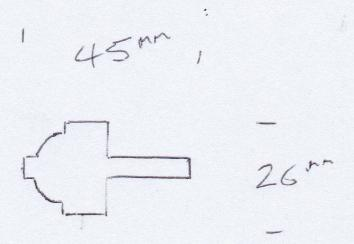
Section of a full size glazing bar for slimlight units
