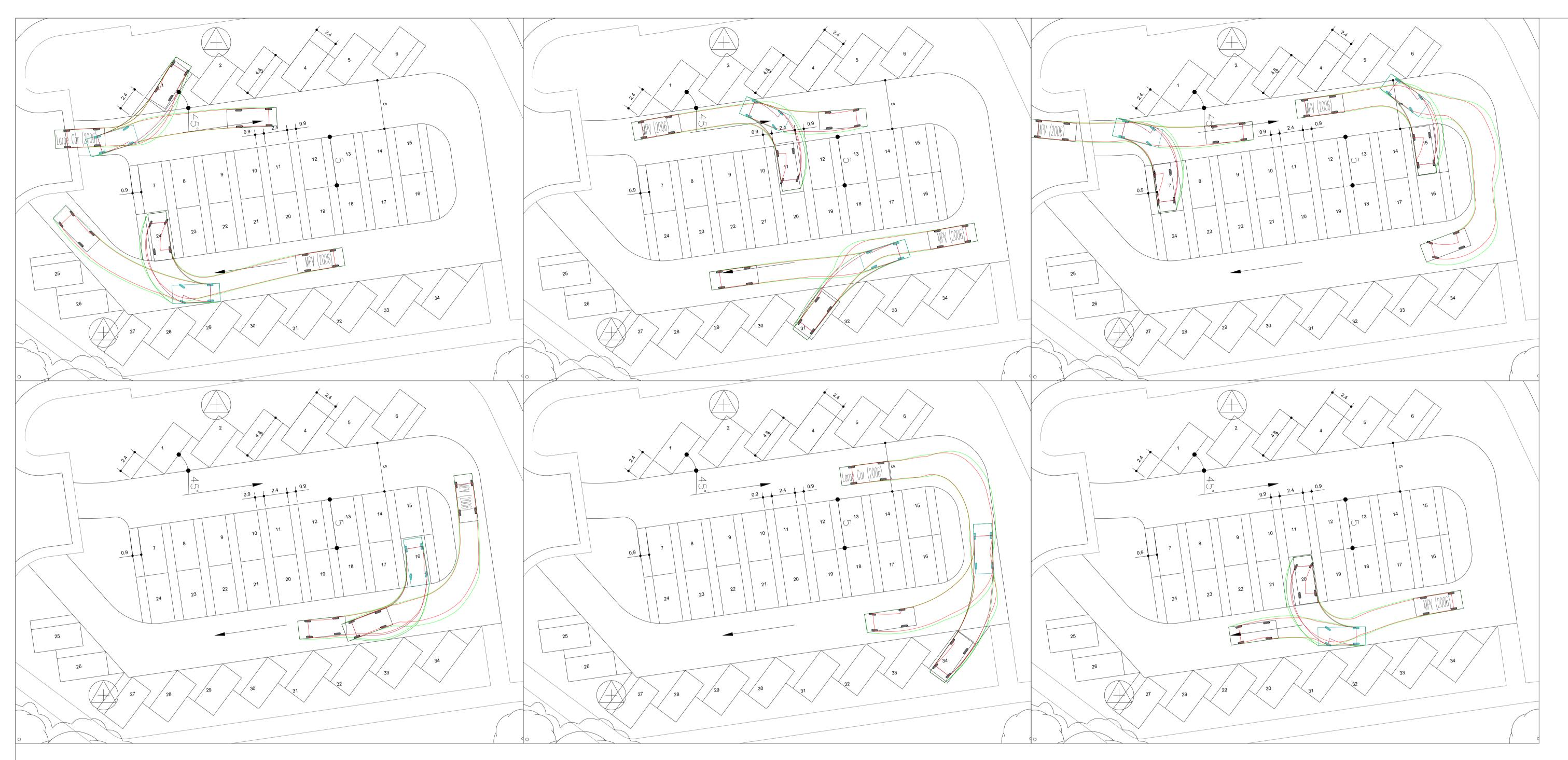
The above tracking are examples for varying plots - for simplistic modelling not parking adjustment maneuvers have been undertaken to 'straighten' car up within bays. This plot shows, however the ability to park and leave the bays in question.
