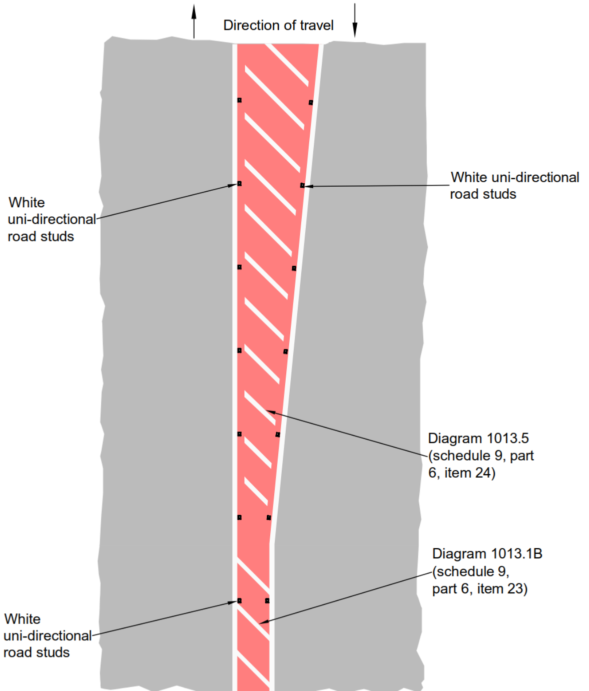
Figure 6.17.1 Interface between TSRGD diagram 1013.1B (shedule 9, part 6, item 23) and 1013.5 (shedule 9, part 6, item 24)
