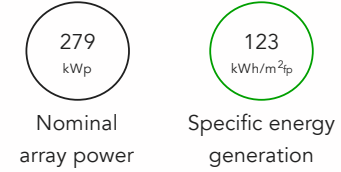
Figure 4.56- Maximising solar generation: 754 x 370W solar photovoltaic panels would enable the school to be energy positive. On an annual basis, it would generate 215% of the annual energy it will consume.
