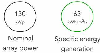
Figure 4.55 - Minimum solar generation for Net Zero Carbon: 384 x 340W solar photovoltaic panels would be sufficient to generate 38 kWh/m 2 /yr and therefore achieve Net Zero Carbon
