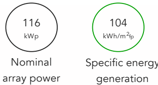
Figure 4.44- Minimum solar generation for Net Zero Carbon: 341 x 340W solar photovoltaic panels would be sufficient to achieve net zero carbon for the modelled unit.
