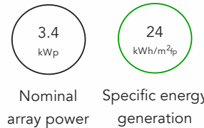
Figure 4.22 - Minimum solar generation for net zero carbon: 10 x 340W solar photovoltaic panels would be sufficient to generate at least 24 kWh/m 2 /yr and therefore achieve net zero carbon (in the case of an air source heat pump heating system).
