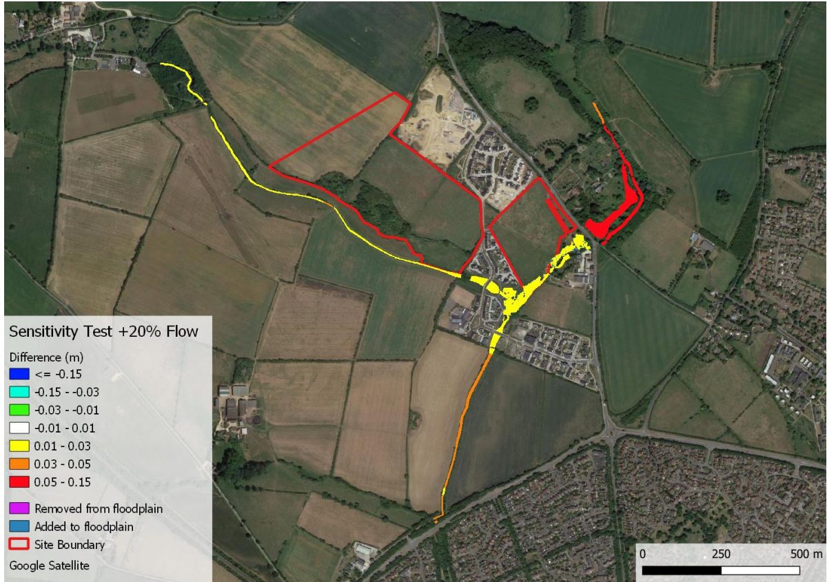
Figure 16: Flow Plus 20% Difference Map
