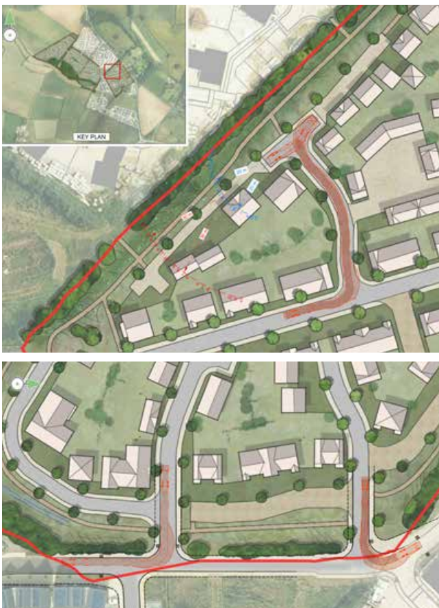
Swept path analysis and refuse drag distance
