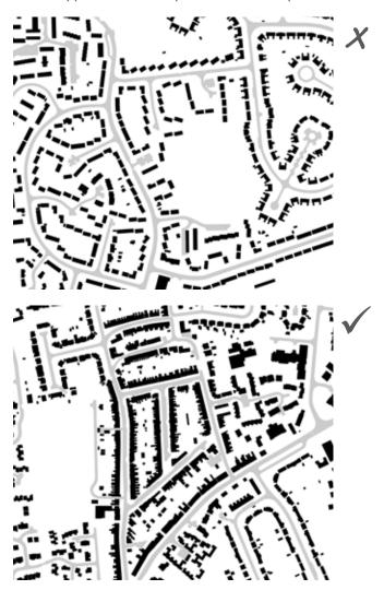
Figure 4.3 Inappropriate dispersed, cul-de-sac and cardependent layout (top) versus traditional, connected, walkable layout (bottom). Both examples from Banbury
