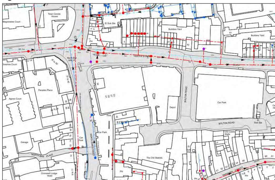
Figure 2.4 – Thames Water sewer asset record
