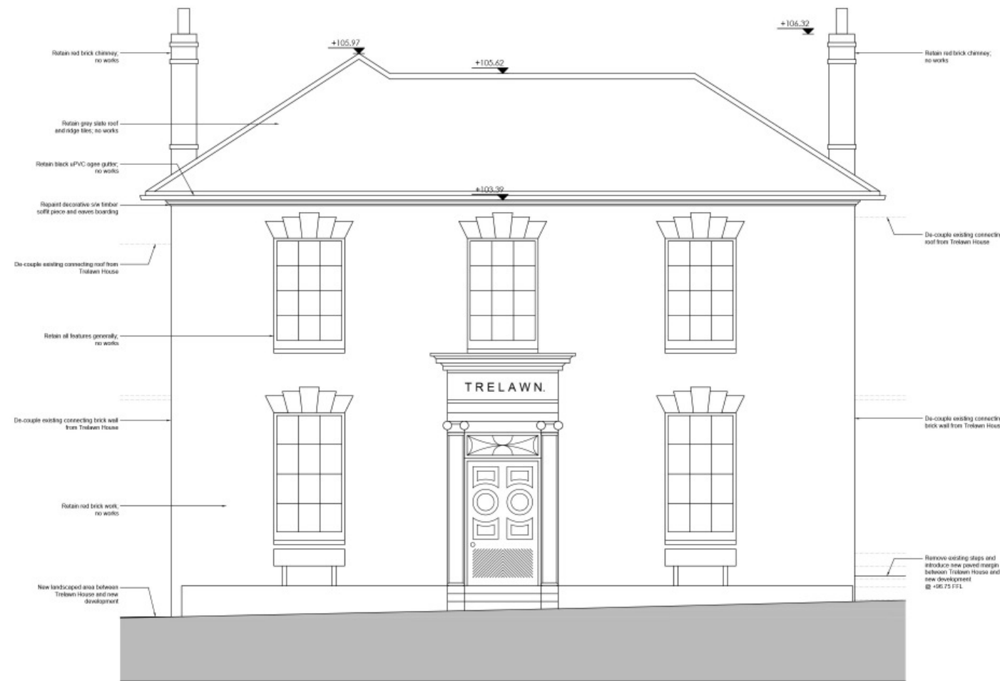
North Bar Street / Western Elevation as proposed
