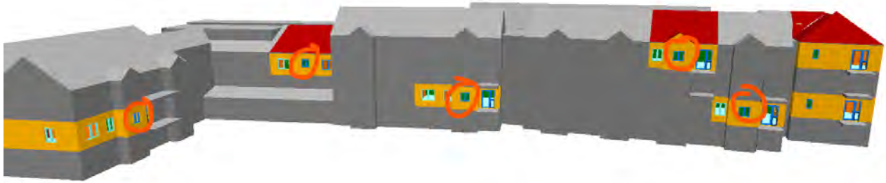
Figure 12. Image indicating the kitchen windows that were reduced to 2 panes
