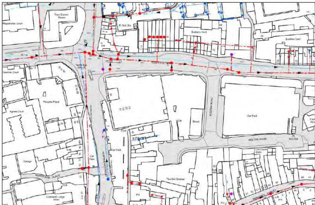
Figure 2.4 – Thames Water sewer asset record
