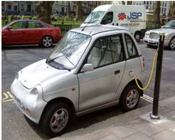
Electric vehicle charging point.
