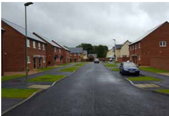
Street currently feels too wide in relation to the height of the buildings but enclosure is to be improved by the planting of street trees, Upper Heyford
