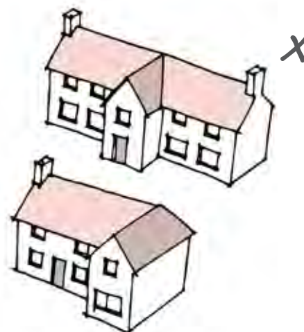
Inappropriate projecting gables
