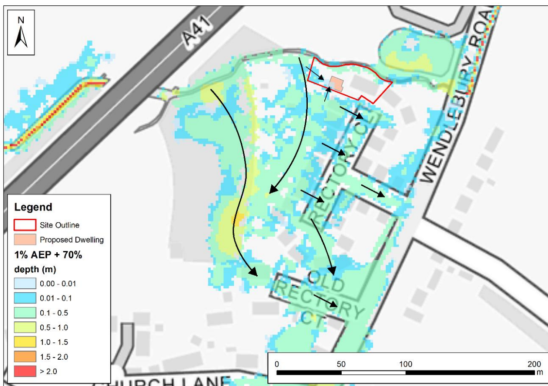
Figure 5-6: Flood mechanism of the Wendlebury Brook during the 1% AEP plus 70% climate change event
