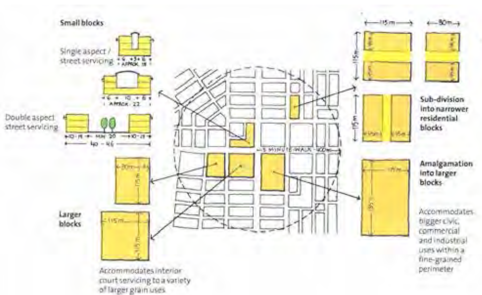
Figure 4.4 Mixed use neighbourhoods should contain a range of block sizes to promote variety (source: Urban Design Compendium p 65, adapted from Baulch, 1993)
