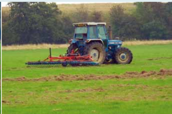
Preparing strips of the ground with a tractor and harrow (spring tine or similar). © RNRP
