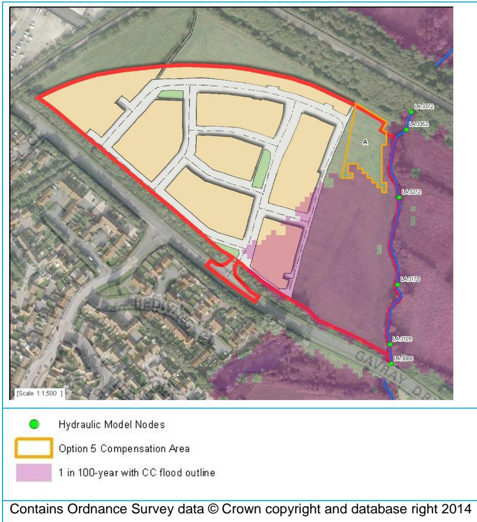
To support the proposed development, it is intended to excavate the proposed floodplain compensation area down to 66.4m AOD, i.e. the minimum ground level observed within zone B. As part of the detailed design phase, deeper and wider excavation works (i.e. for landscaping purpose or to enhance hydraulic connectivity with the main channel) may be considered however their associated volumes were not considered in the floodplain compensation calculations.
