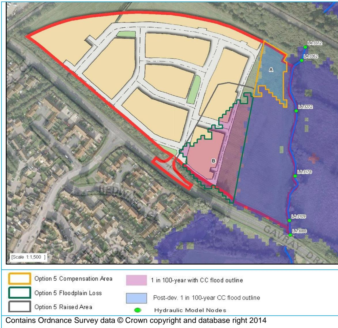
The pre-development flood extent shows flooding across the site as would be expected prior to raising the ground levels within the residential area. The floodplain compensation event shows the additional capacity made available along the Langford Brook's right hand bank, in the north eastern corner of the site.
