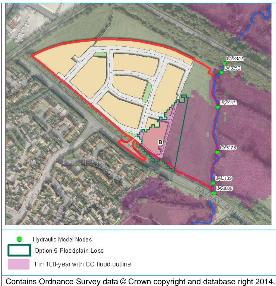
Using a Digital Elevation Model (DEM) representing ground levels within the site boundary and in-house GIS tools, a level-area-volume relationship was derived for the extent represented by zone B. Results are indicated in Table 6- 1.
