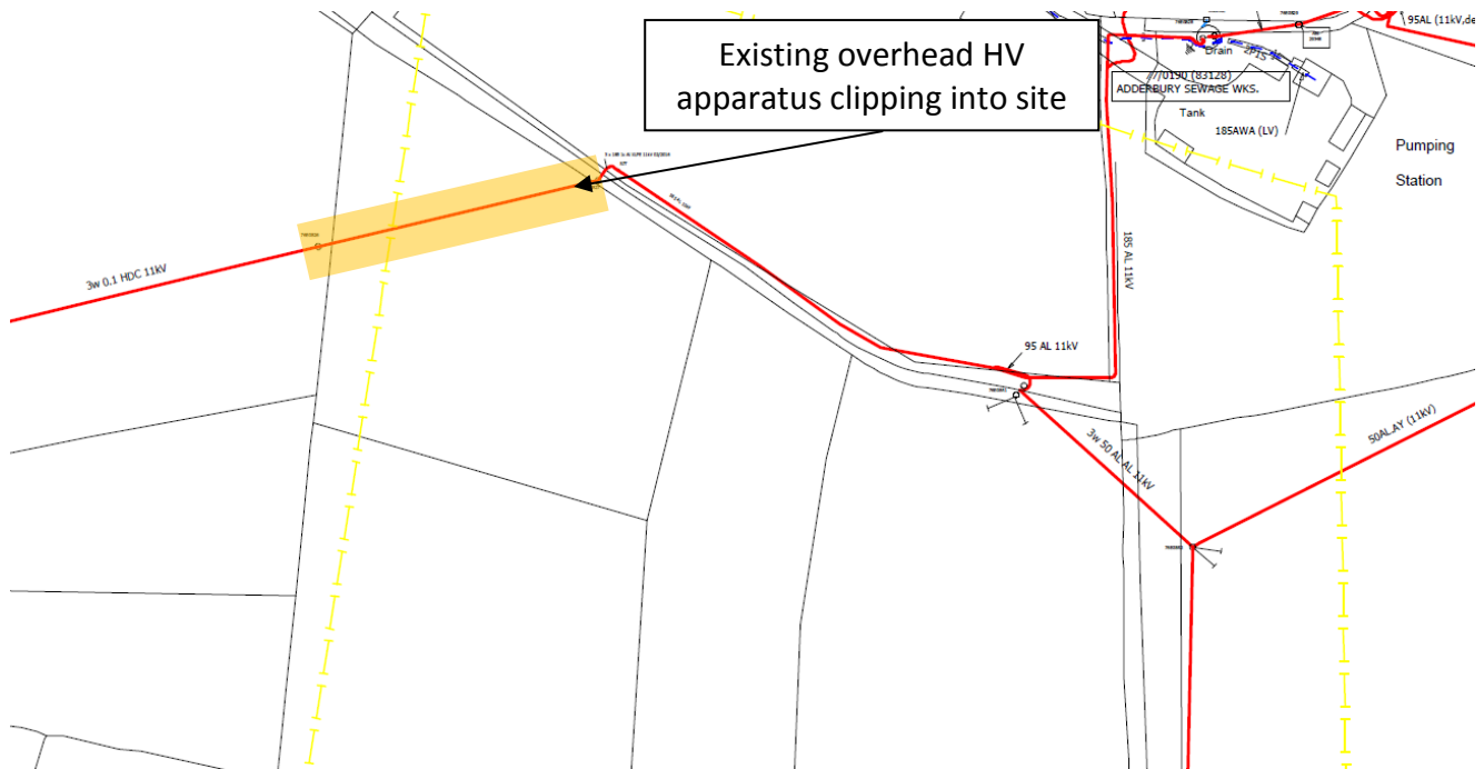
Figure 2.3 – Existing overhead HV apparatus clipping the northern boundary of the site assumed to be retained in greenspace upon the northern boundary.
