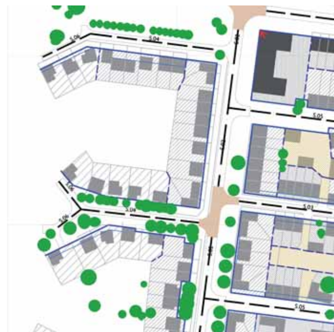
fig. 4.27 An extract from the regulating plan showing controlling lines and plot series
