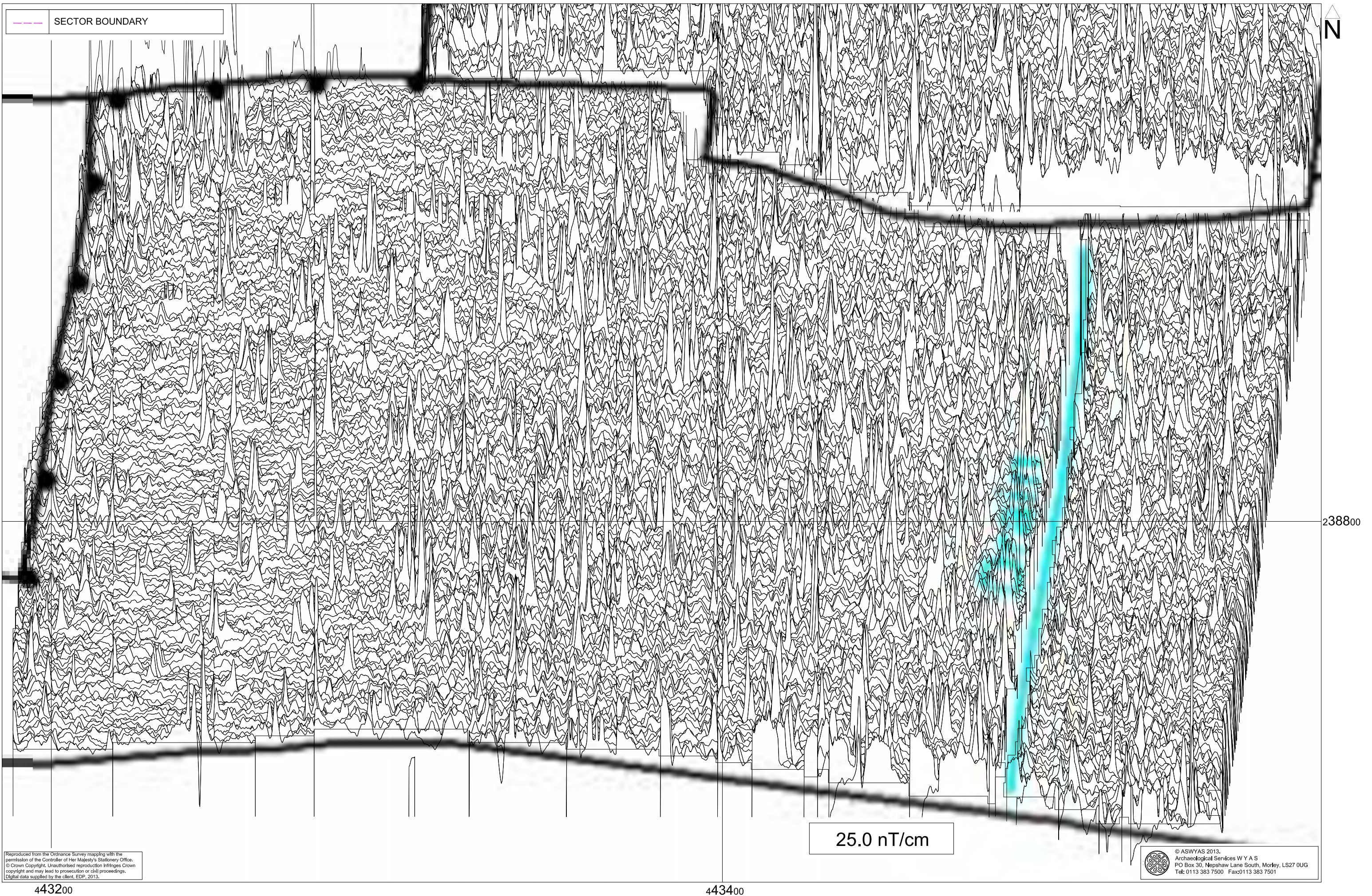
Fig. 30. XY trace plot of minimally processed magnetometer data; Field 9 and Field 10 (1:1000 @ A3)
