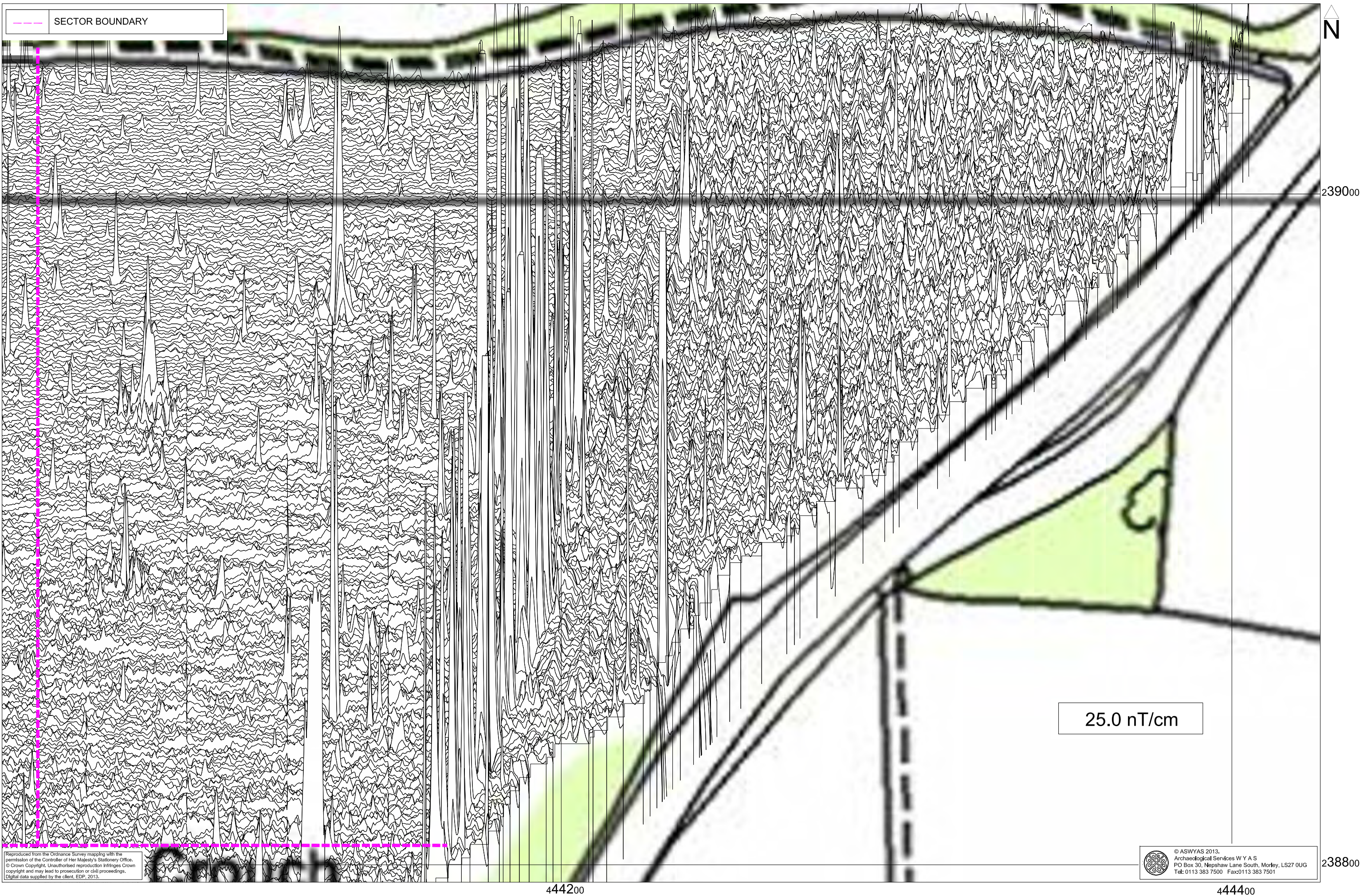
Fig. 12. XY trace plot of minimally processed magnetometer data; Field 3, Sector 2 (1:1000 @ A3)
