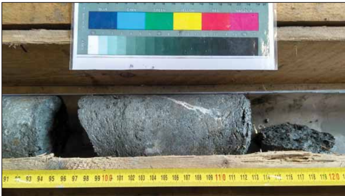
BH2, 10.00-10.10m, calcite veins near base of Cornbrash Formation
