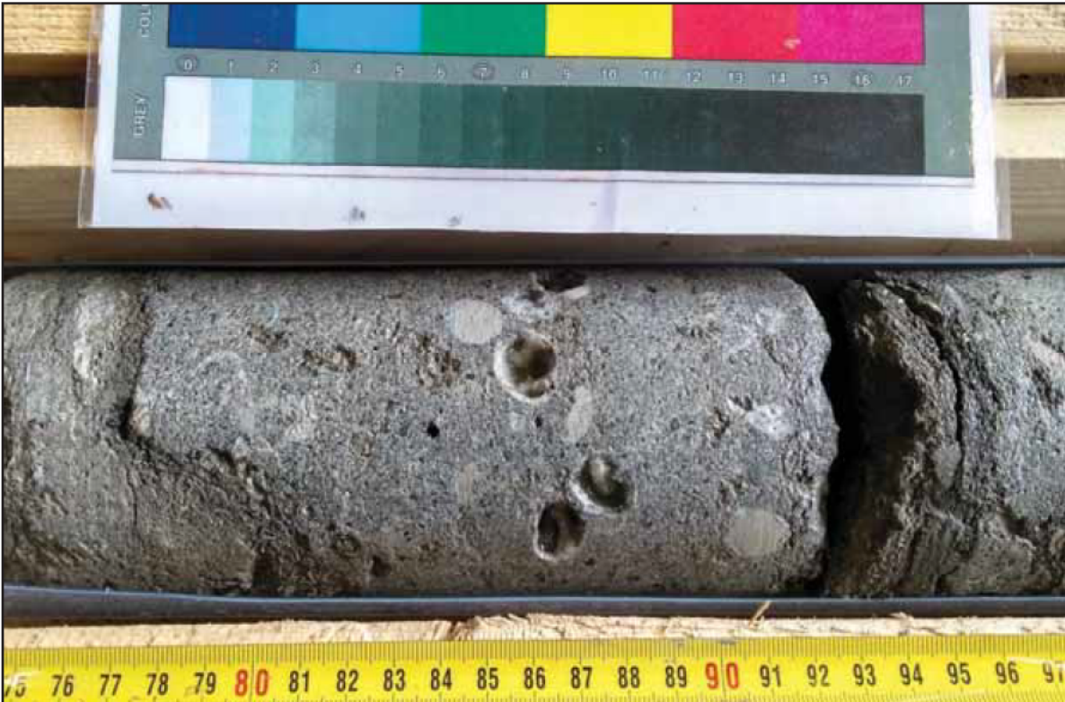
BH1, 9.75-10.00m, example of calcite-filled bivalves in Cornbrash Formation
