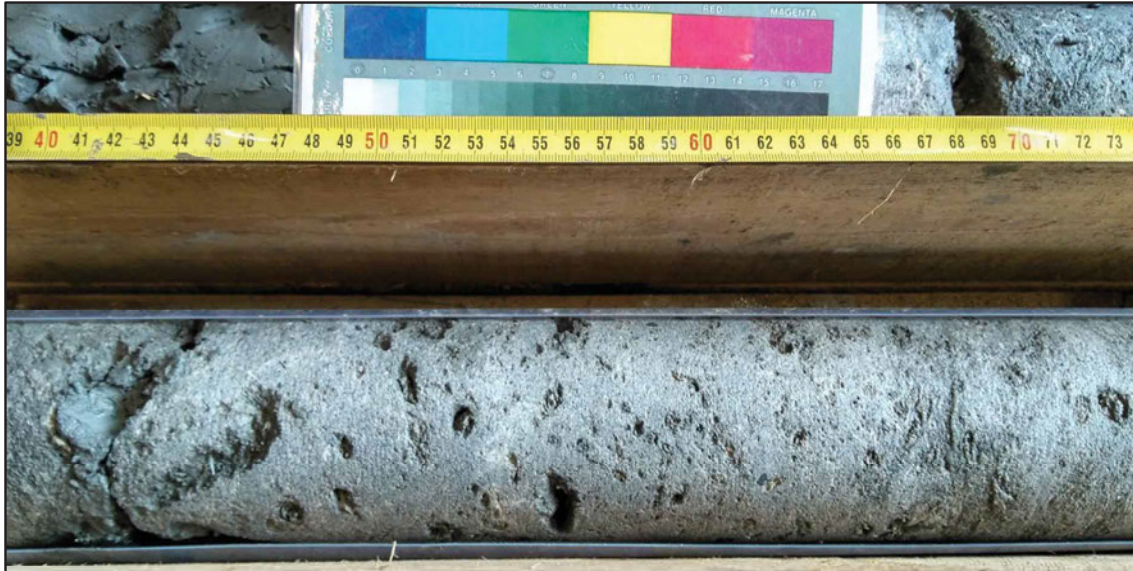
BH3, 10.40m-10.70, bioturbation/bivalve burrows in Cornbrash Formation.
