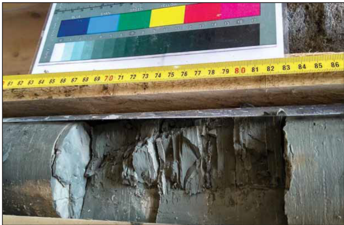
BH1, 11.60-11.85m, example of laminae and 'ripples' of light grey and white silt in very stiff, laminated, green grey clay of the Forest Marble Formation.
