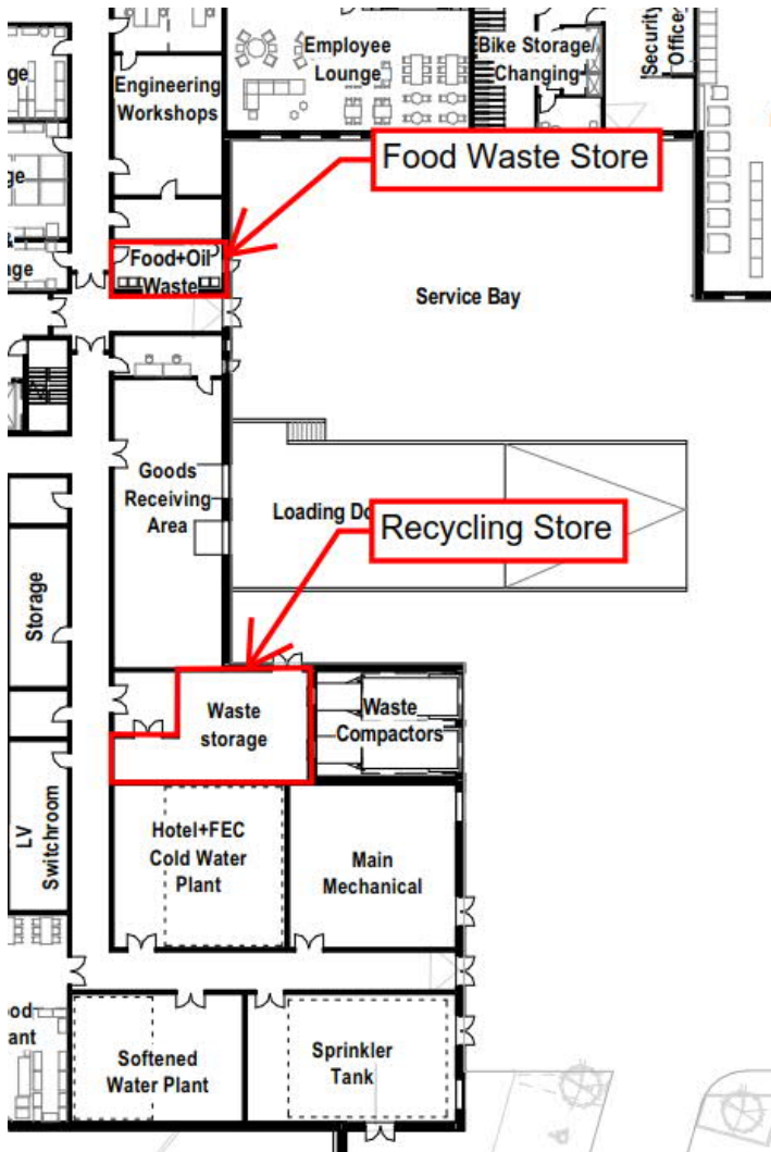
Figure 3-6 - Locations of food waste store and recycling store (refer to Appendix for full ground floor plan)
