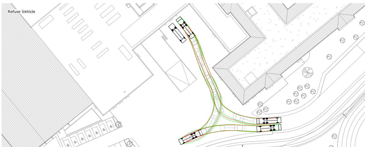
Source: Motion; Great Wolf Resort, Bicester, Swept Path Analysis Deliver Yard; Drawing No. 803047-TK58
