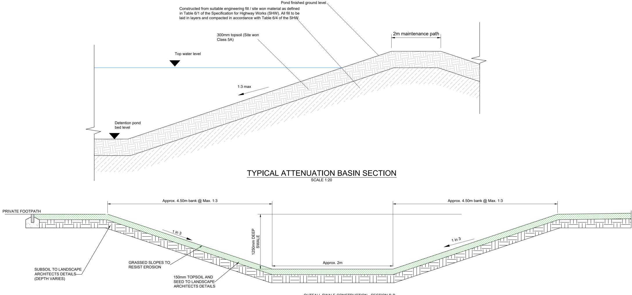
OUTFALL SWALE CONSTRUCTION - SECTION B-B SCALE 1:20
