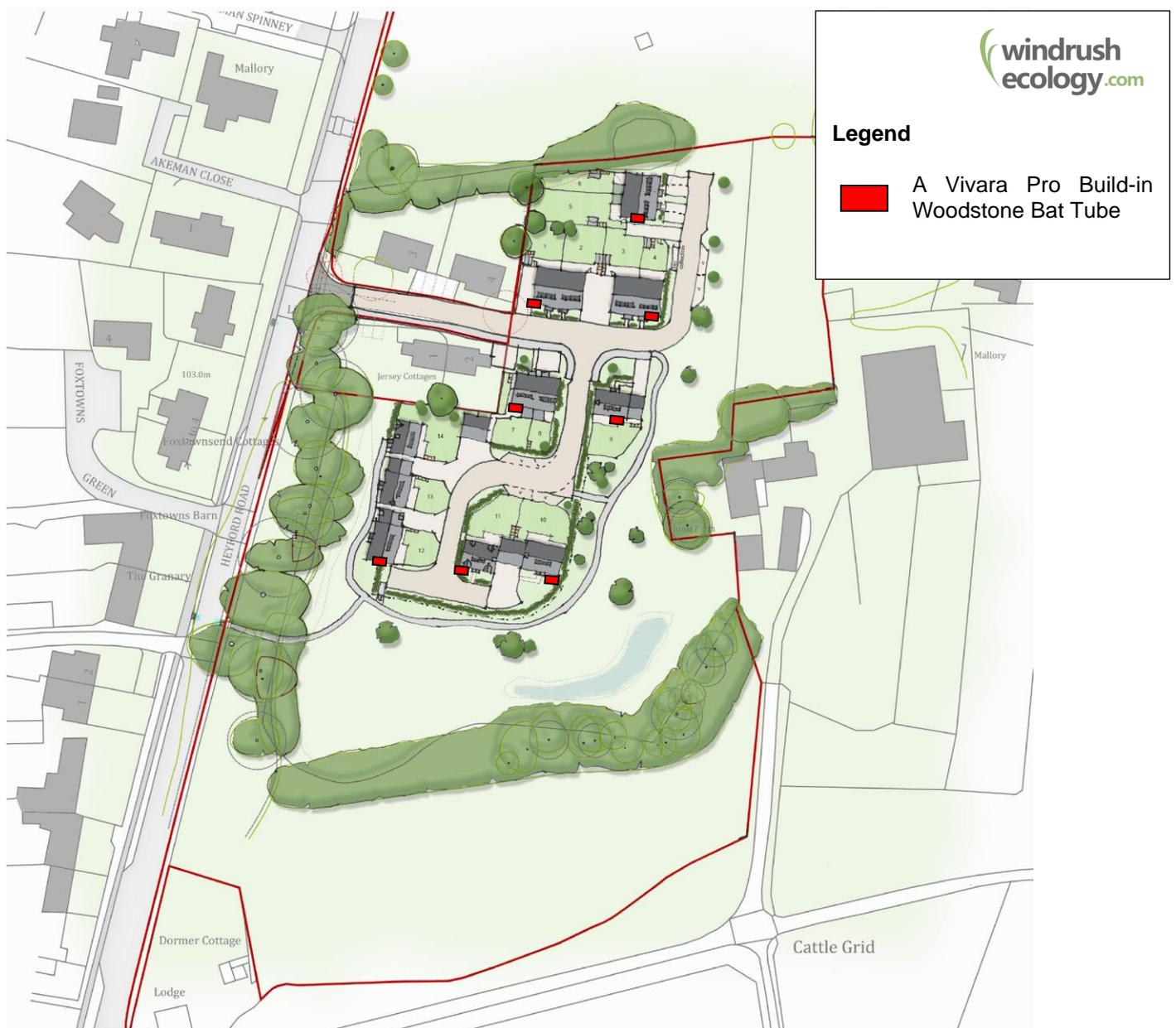
Figure 7. Plan showing the location of the bat tubes.
