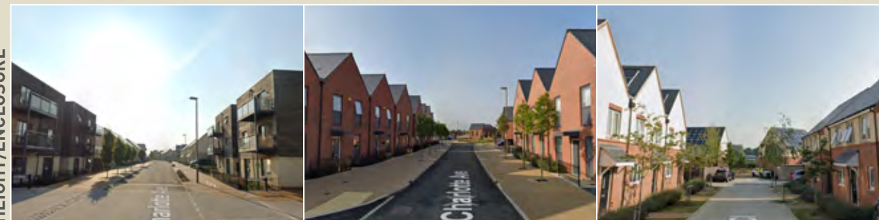
2-3 storey to primary streets with taller buildings located at key junctions. 2 storey continuous frontage with minimal set back provides a strong sense of enclosure. Narrower carriageway and wider pavements with trees provide a more pedestrian friendly street. 2 storey dwellings close to the carriageway along shared surface secondary streets provide a good sense of enclosure.
