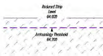
Topsoil Strip (Stage 1) 1:25
