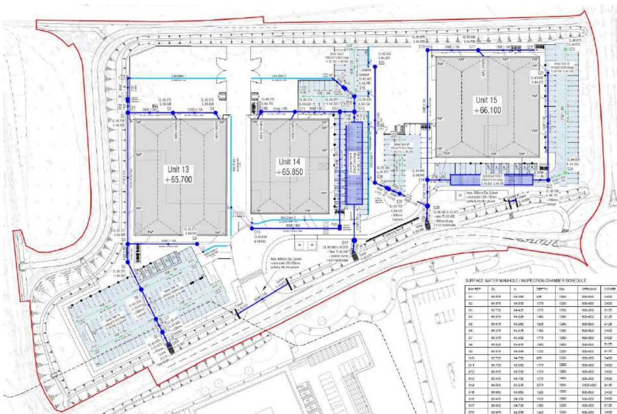
Figure 5-2 – Extract of Drainage Scheme
