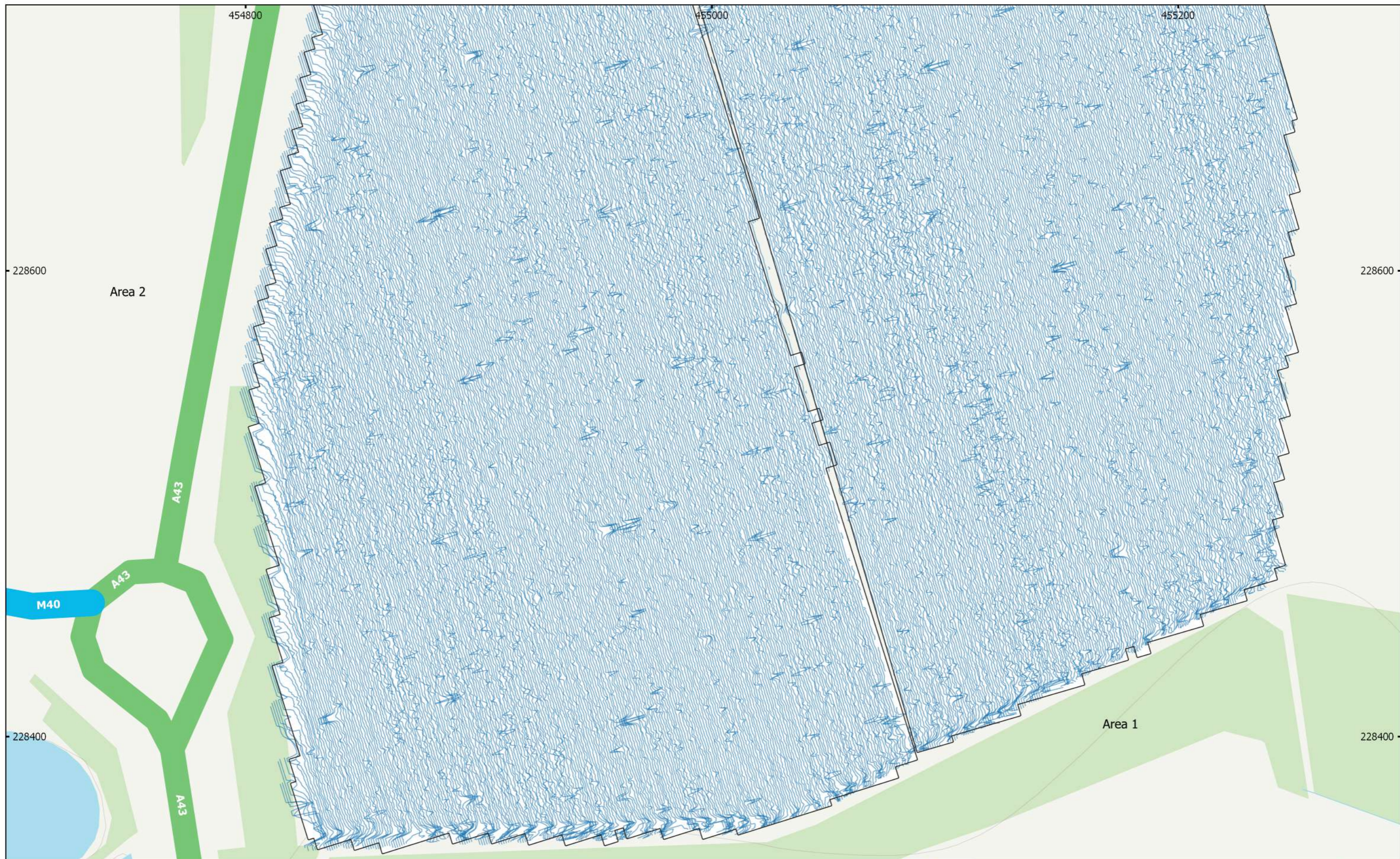
MSSP963 - J10, M40, Baynard's Green - Area to east of A43 Figure 10 - XY Trace Plot (South) 30nT/cm at 1:1,500 @ A3 Copyright Magnitude Surveys Ltd 2021 Contains Ordnance Survey data © Crown Copyright and database right 2021
