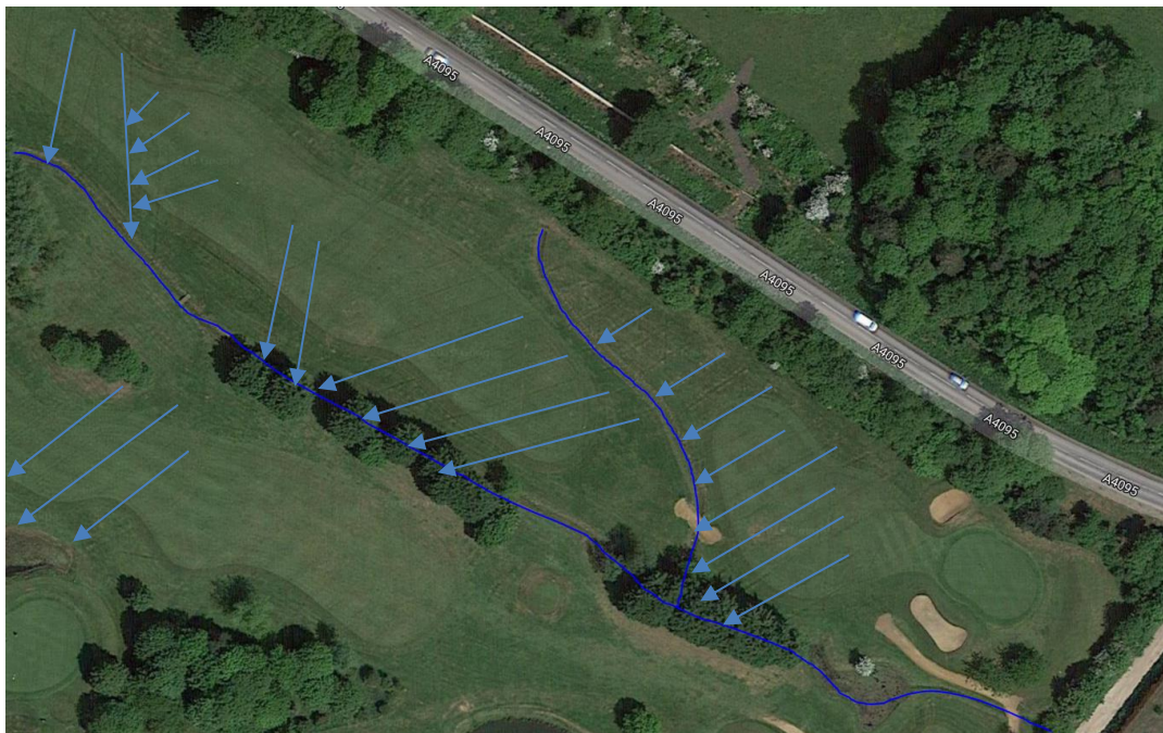
Figure 3-4: Aerial Imagery Showing Land Drainage
