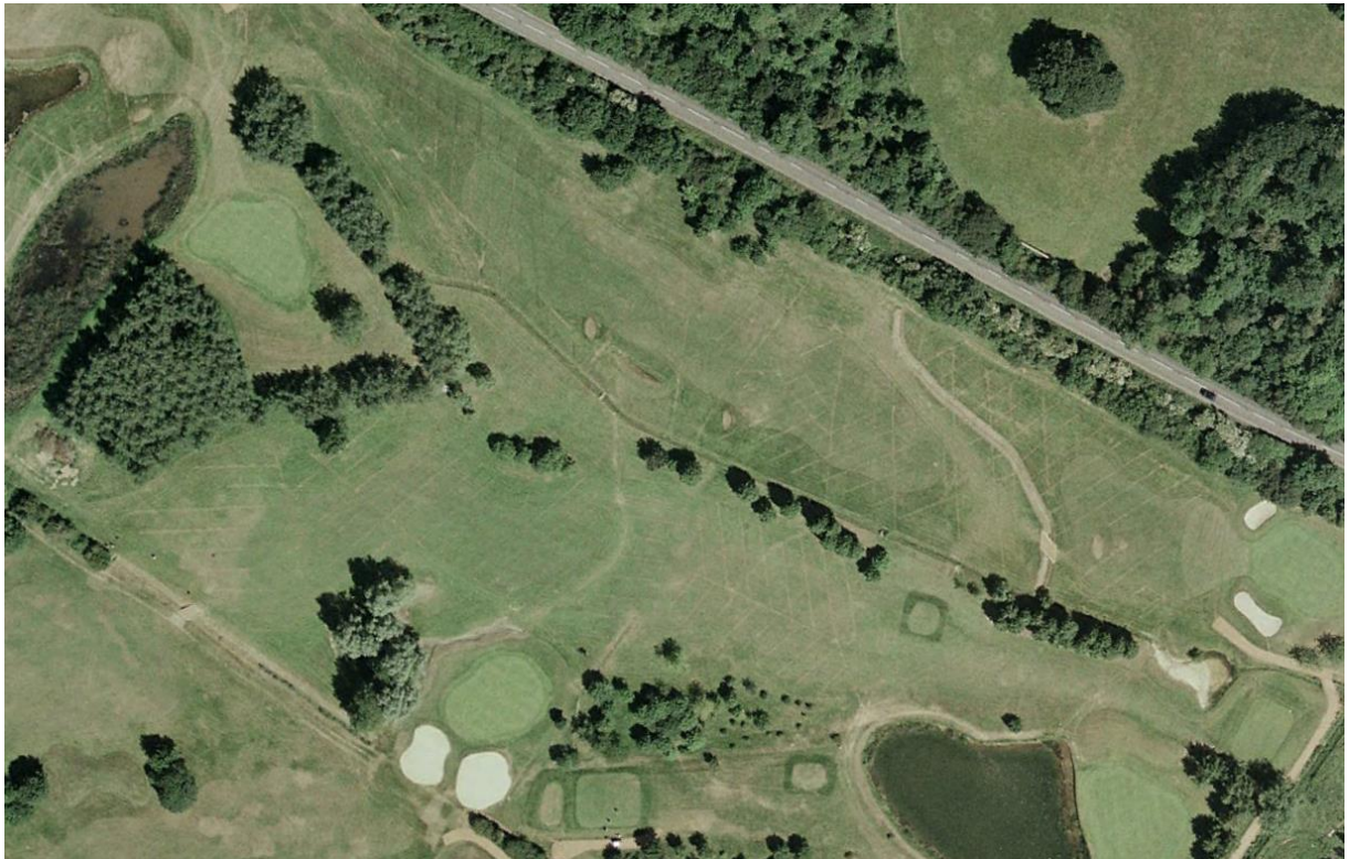
Figure 4-4: Aerial Imagery Showing Evidence of Land Drainage
