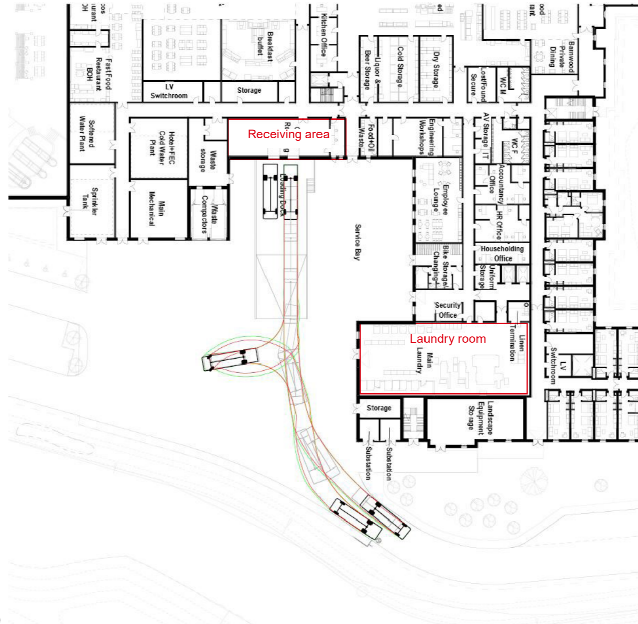
Service delivery area sketch diagram. Swept Paths as per Motion consultant's drawing: 1803047-TK44A & 1803047-TK56
