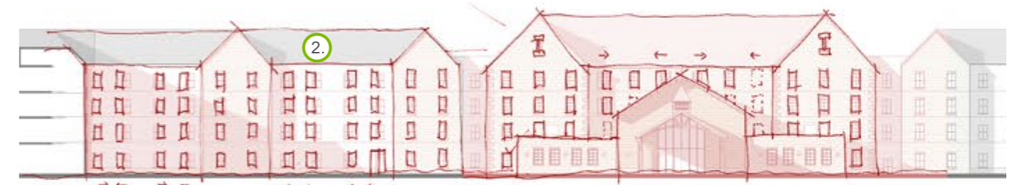
Windows repositioning on front, north east elevation.
