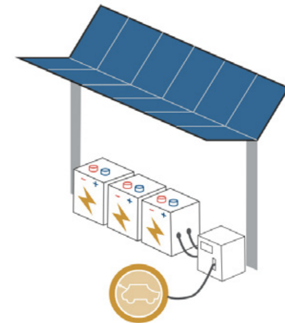
EV charging hub collocating battery storage and PV
