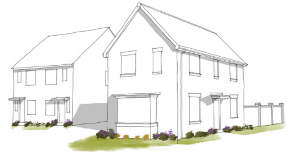
Corner turning dwellings enhanced by bay windows and/or change in materials and their application
