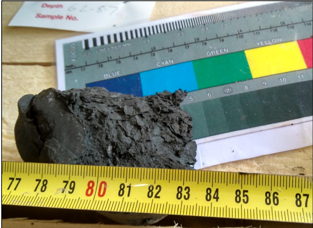
BH4, 6.80m, example of close fissures in Kellaways Clay Member
