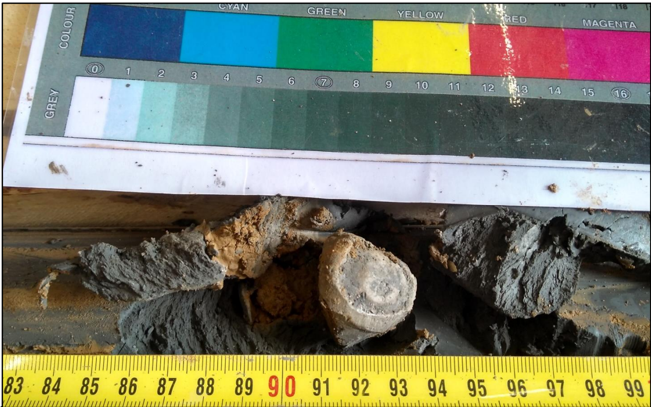
BH2, 5.00m, coarse gravel size concretionary limestone nodule in Kellaways Clay Member
