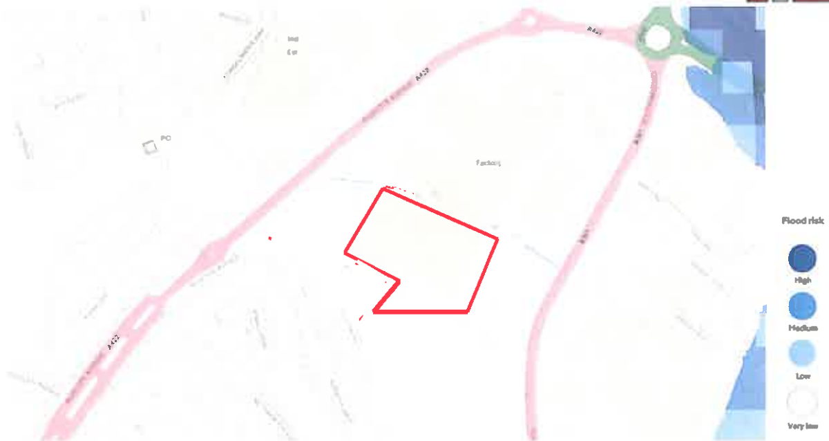
Figure 5.1 - Environment Agency Online Flood Map Extract (Approximate Site Extents Edged Red) - Flood Risk from rivers or the sea.
