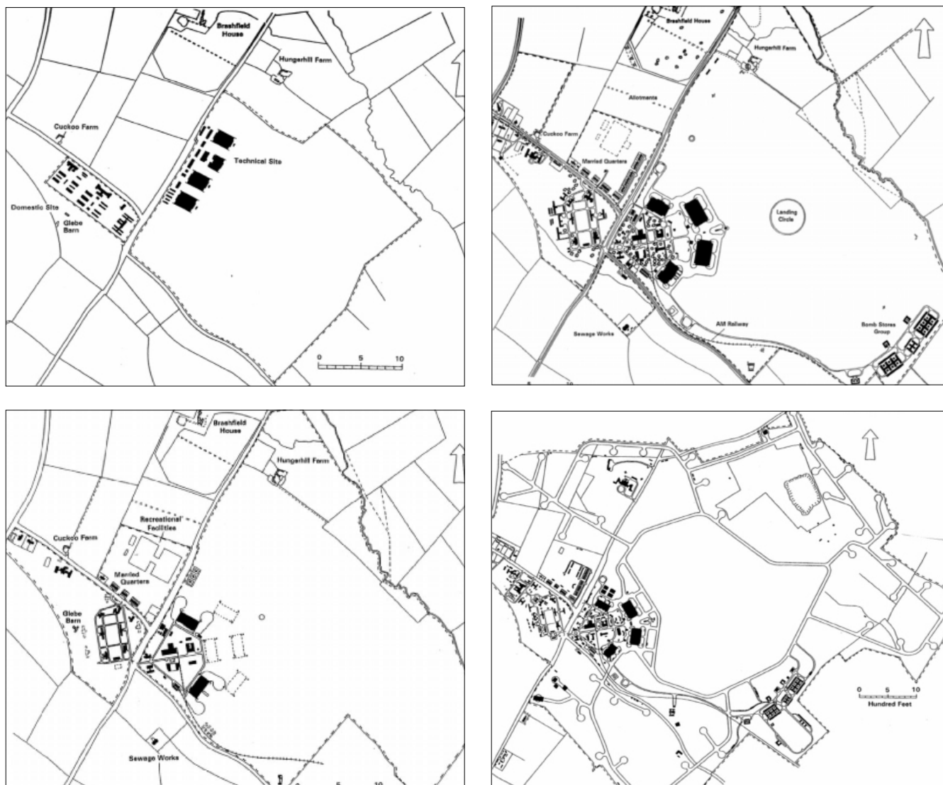
Fig 6: Map regression (1918-1945) illustrating the development of the airfield, domestic and technical site . Particularly noteworthy are the 1918 and 1926 OS Maps whose comparison highlights the marked and dramatic impact of Trenchard's philosophies (enacted from 1925 onwards) on the physical layout of both the domestic and technical site. The site's WWI incarnation with linear siting of its buildings is replaced by a trident layout characterised by a dispersal of structures. The later (1939 and 1945) maps evidence how the site becomes further populated with structures as its functional requirements evolved - with the need for instance for the introduction of defensive structures during the war period. 5
