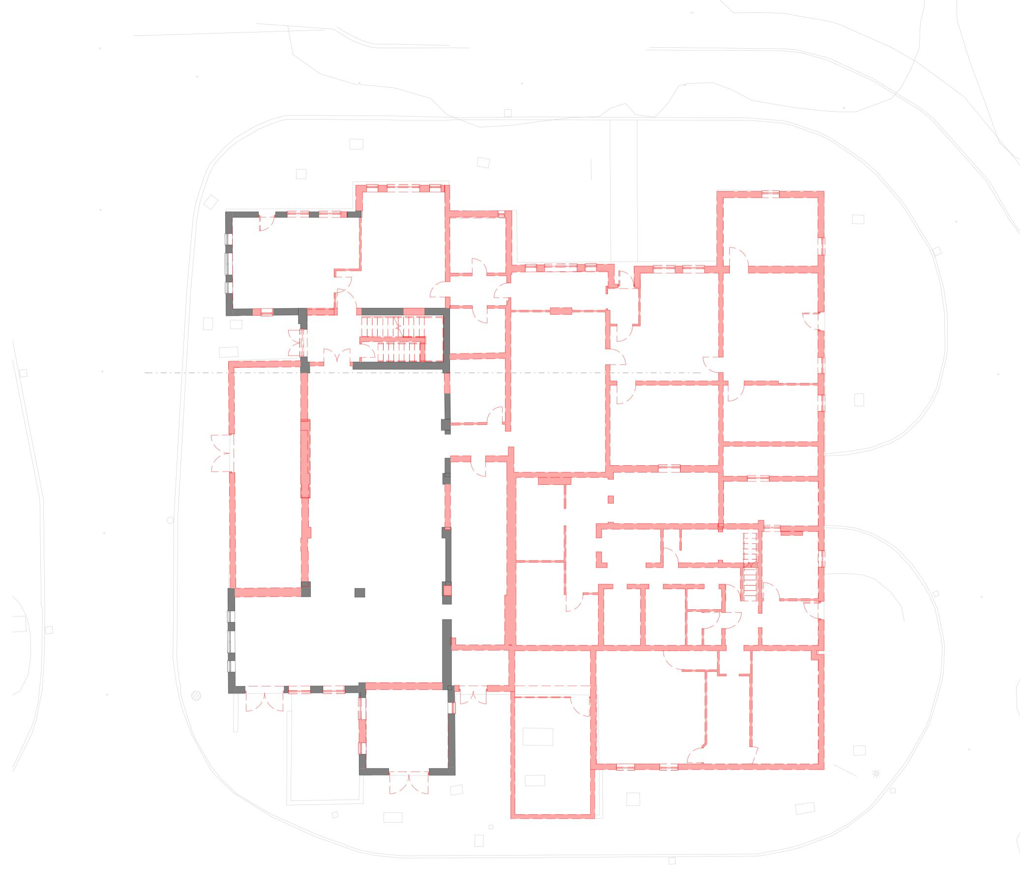
Building 455 - Demolitions Ground Floor Plan
