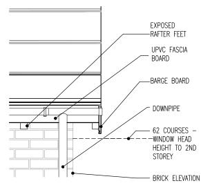
EXPOSED RAFTER FEET EAVES, BARGE BOARD & VERGE DETAIL STONE ELEVATION SCALE 1:20 ROOF PITCH VARIES
