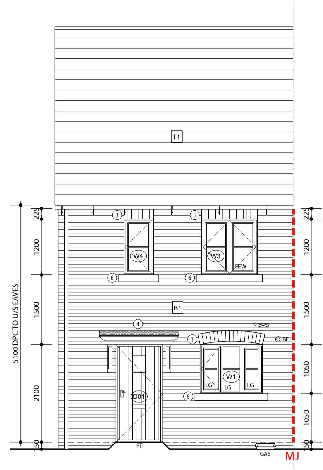
FRONT ELEVATION EE1 - BRICK PLOTS, 82 (AS) - 29, 96 (OPP)
