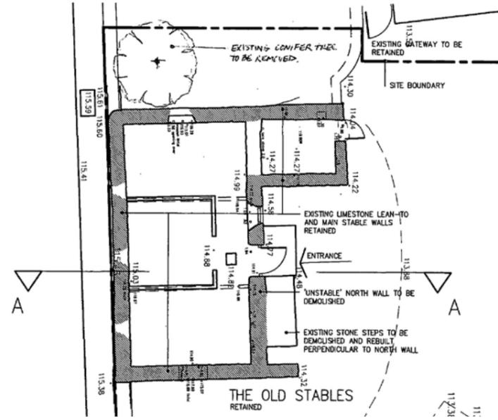
Fig.8 - The Old Stables Manor Farm Existing Ground Floor Plan
