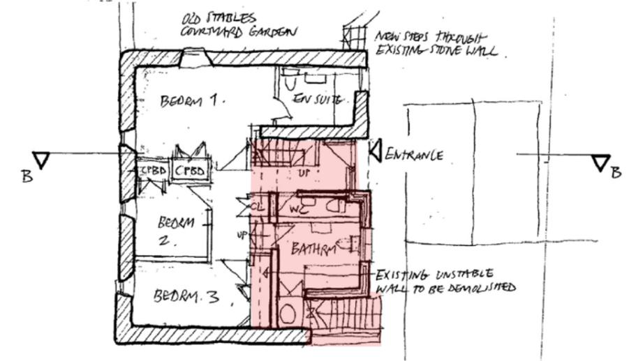
Fig.9 - The Old Stables Manor Farm Proposed Ground Floor Plan
