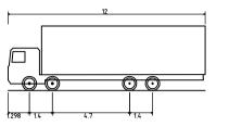
Rigid Truck with Wing Mirrors Overall Length Overall Widfh Overall Body Height Min Body Ground Clearance Track Width Lock to Lock Time Kerb to Kerb Turning Radius
